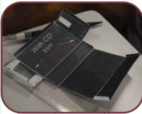
Fig. 11: Cut and assemble the spectroscope, leaving the black part inside.
