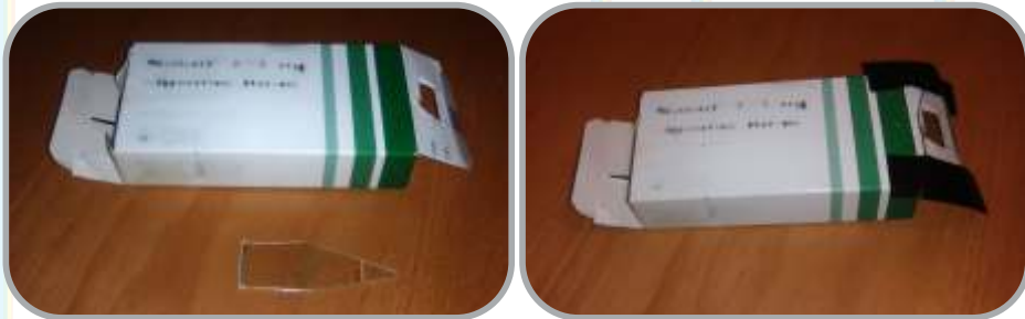
Fig. 19: Spectroscope with a medicine box and a piece of CD. It is simpler but we cannot measure wavelengths.
